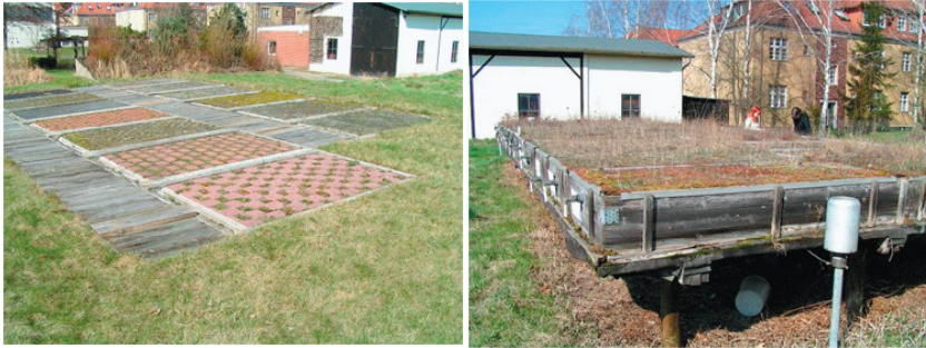
Figure 8+9. Lysimeterstation at the same place for measurements of the hydrology of semi permeable surfaces (left, coloumn 3-5 of figure 5) and evaporation and runoff of extensive greened roof plots (right, coloumn 6-7 of figure 5), TU Berlin in Berlin-Wilmersdorf
