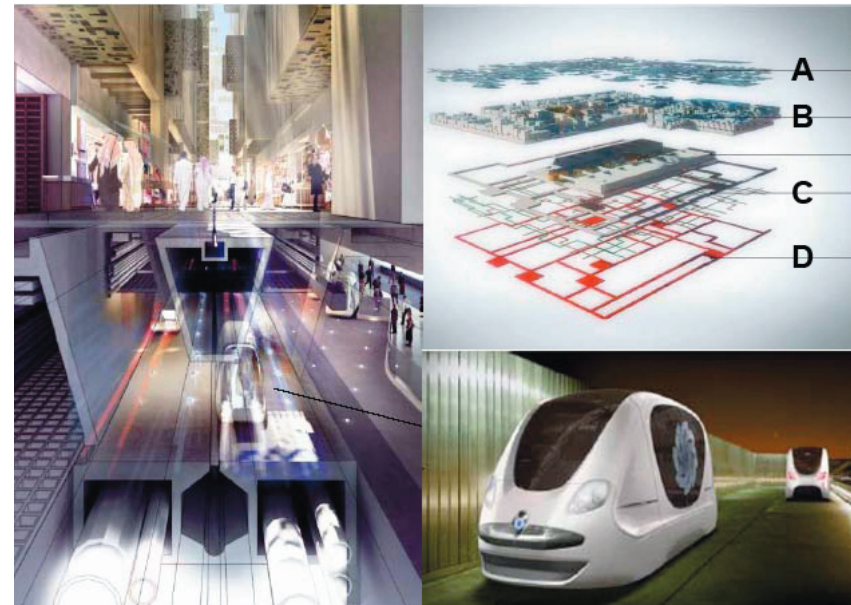
Figure 2.26 Artistic rendition of underground PRT system, PRT cars and infrastructure layers. A) PV roofscape, B) residential, commercial and light rail system C) secondary infrastructure, PRT and raised street network D) primary infrastructure (Hahn, 2009).
