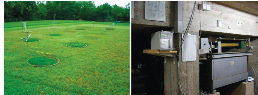
Figure 6+7. Lysimeterstation at the Technische Universitaet in Berlin-Wilmersdorf, measurement of precipitation, evaporation and percolation (groundwater recharge), surface (left) and balances in the underground (right, colour 1+2 of figure 5)
